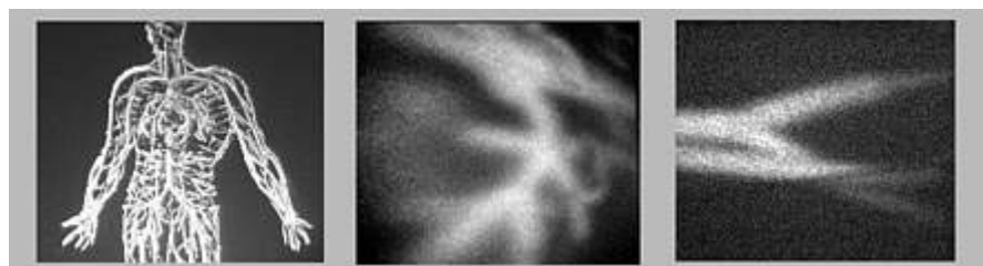
Figure 5. Traditional H2 hologram projection of the image, A projection of the image, B1) Illuminating spot size 1 mm, projection screen distance 50 cm, picture width 30 cm, B2) Illuminating spot size 0.2 mm, projection screen distance 50 cm, picture width 30 cm.
