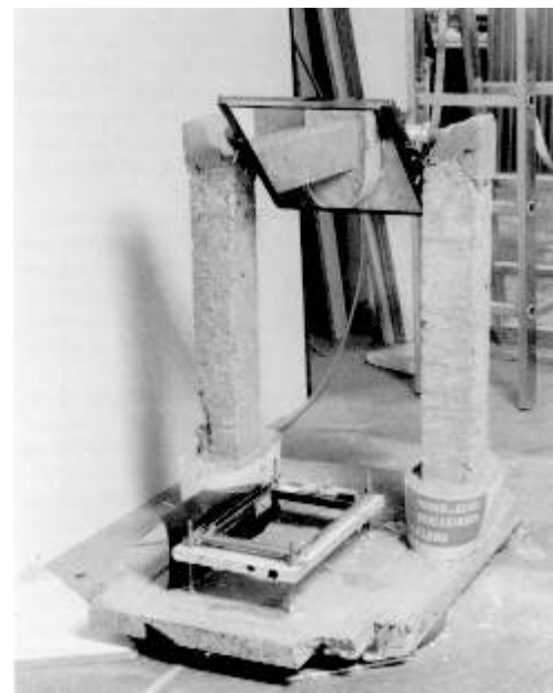
Fig. 2. This shooting surface and overhead mirror rig, created from an old stone kitchen table and a broken concrete fence pole, was used in the author's homemade holography lab in a shed behind his house in 1980.
