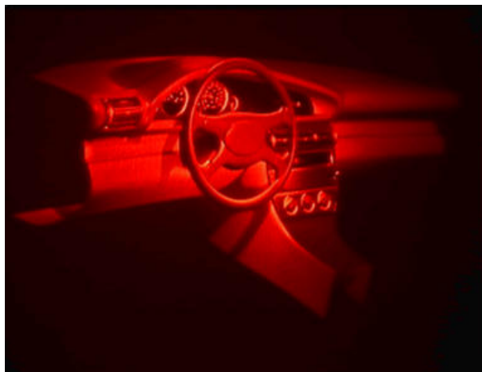
Fig. 11.(a) Computer-assisted design (CAD) drawing of a dashboard and (b) a rendering of the dashboard using 3D animation software TRACES, 1994. Images designed in TRACES can be automatically transferred into photoresist masters from which the embossed holographic material, e.g. stickers, are produced. The photoresist records the graphic computer data from an LCD screen. With this new LCD technique, pixels are visible, comparable to 35mm slide film quality.
